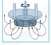
The combined intake and expulsion of ingredients sets up a circulatory mixing pattern within the vessel. In a short time all the ingredients pass through the workhead and dispersion is completed. The dispersed phase is added to the vessel and an emulsion is rapidly formed. Particle size is progressively reduced, producing a stable and homogeneous mixture.
