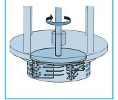
The powdered ingredients are de-agglomerated in the clearance between the ends of the rotor blades and the stator wall, becoming fully dispersed. The product is forced out through the stator at high velocity and returned to the mix, as fresh ingredients are simultaneously drawn into the workhead.
